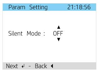
This function is usually used during the night, so that ventilation does not disturb users when they sleep.
