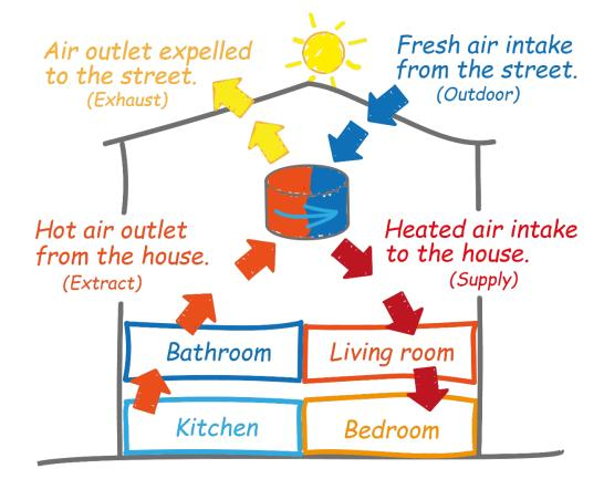
The LYNX heat recovery units, have an intelligent software that measures and adjusts the flow and temperature of the air, the CO2 level and the relative humidity in the environment, all this added to the rotor offers users an automatic ventilation system that controls thermal efficiency and the air quality.
