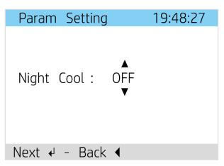
Night Cool Point, this feature is used to define the temperature desired by the user. It can be set from 16°C to 26°C which will regulate the incoming air temperature.
