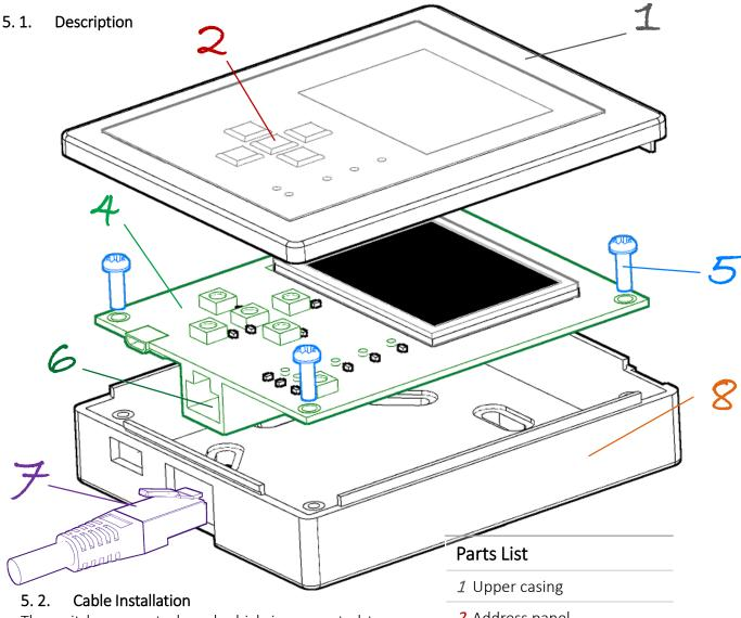
The unit has a control cord which is connected to the control panel to access the unit. It is important that this plug is easily accessible afterwards for possible faults or when changing the unit.
