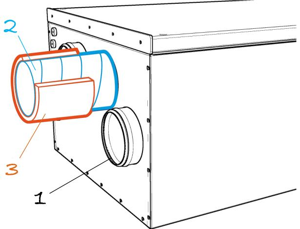
To install the spiral pipes [2], pull them down towards the niple [1] until they reach the case of the unit, then cover the tube with the insulation. Make sure there is no gaps between the insulation and the unit in order to avoid condensation and possible formation of ice.
