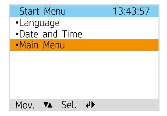
Once the unit has started, on the control panel go to: Main Menu / Advanced user / Calibration Test.
